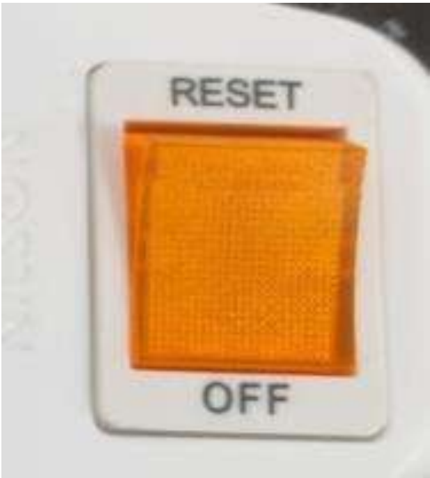
Photo 8. Circuit breaker with pilot light (enclosure)
